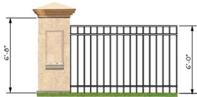
C ORNAMENTAL METAL FENCE WITH COLUMN TERMINUS
