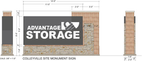
COLLEYVILLE SITE MONUMENT SIGN - Materials to match building - Sign comprised of reinforced dark bronze face, letters and images are cut in relief with white lexan laminated behind. Backlit with LED.
