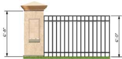
C ORNAMENTAL METAL FENCE WITH COLUMN TERMINUS
