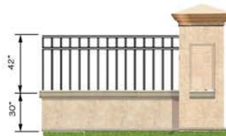
D LOW STONE WALL WITH ORNAMENTAL METAL FENCE
