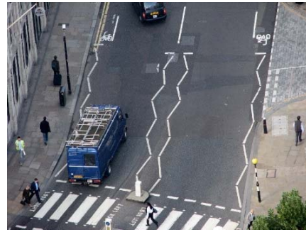
Figure 3: Zig-Zag Pavement Marking Example 2
