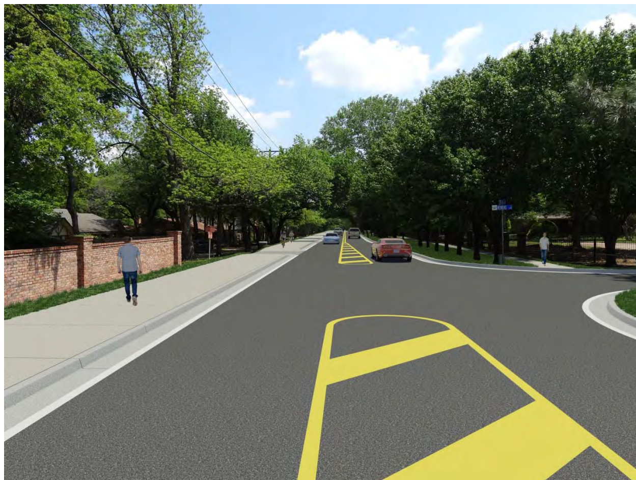
Barrier Curb with Sidewalk Adjacent
