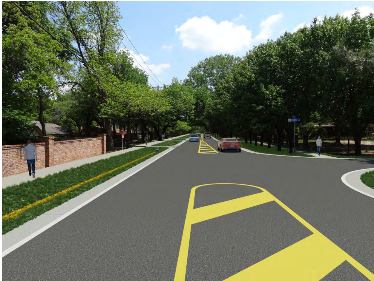
Ribbon Curb with Swale
