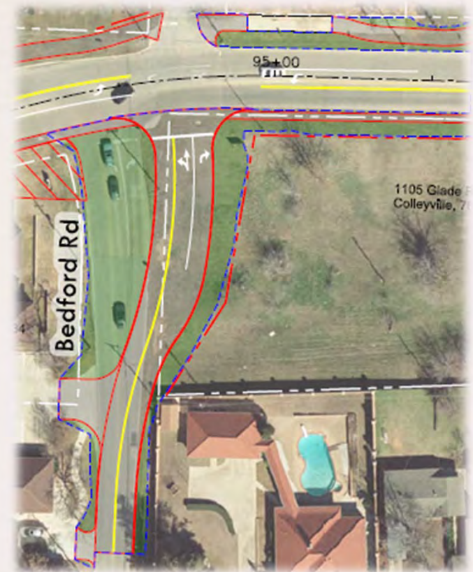
Realignment of Bedford Road Intersection
