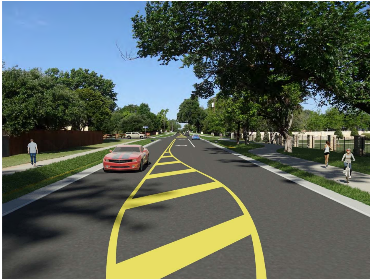
Ribbon Curb with Swale
