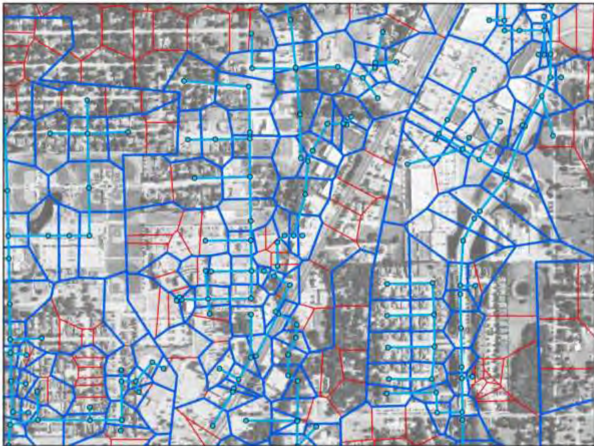
Figure 38: Dissolved Thiessen Polygons Based on Model Manholes and System Connectivity
