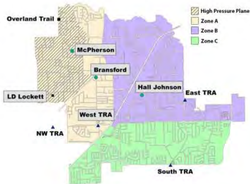
Figure 1 – Pressure Plane Distribution
