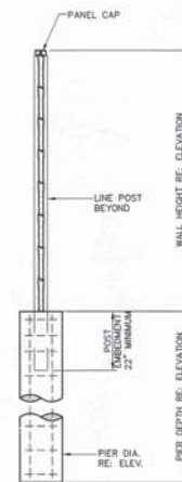
SECTION - SCREENING WALL
