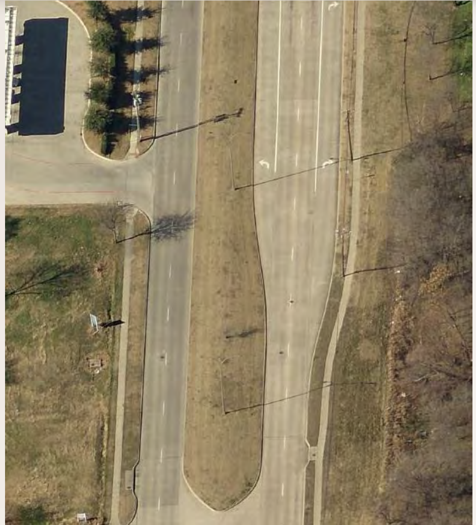
Four Lane Section Expanding for an Intersection
