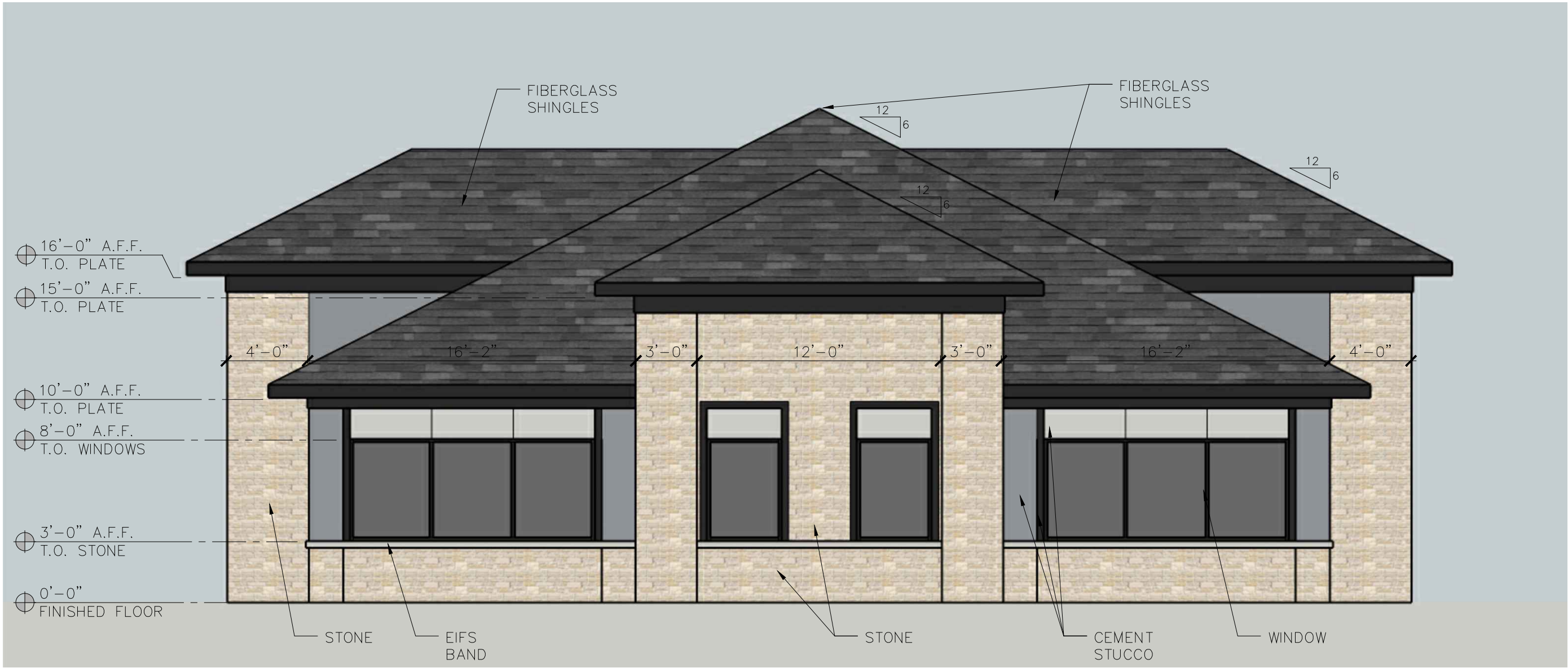
1 BUILDING A - WEST ELEVATION SCALE: 3/16" = 1'-0"
