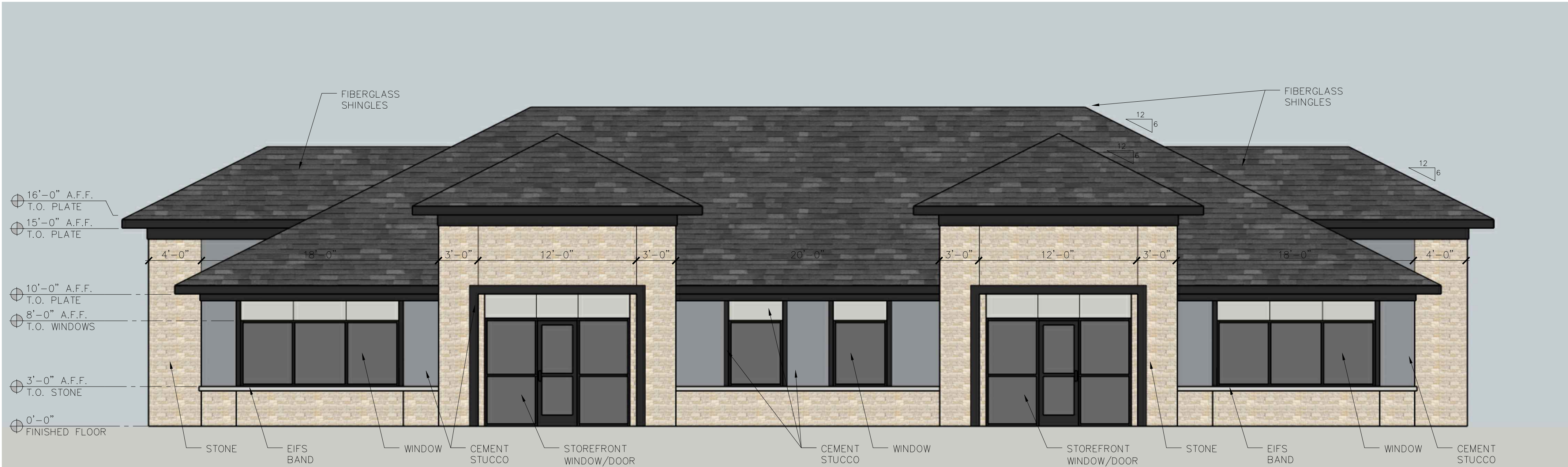
2 BUILDING A - SOUTH ELEVATION SCALE: 3/16" = 1'-0"
