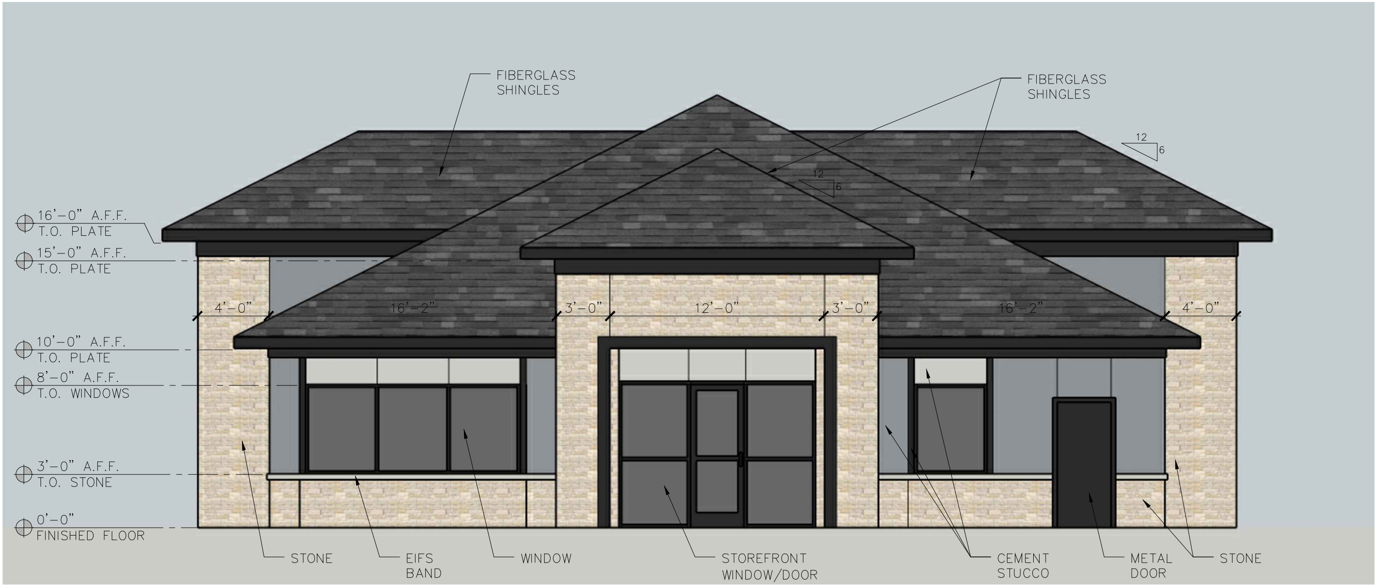
1 BUILDING A - EAST ELEVATION
