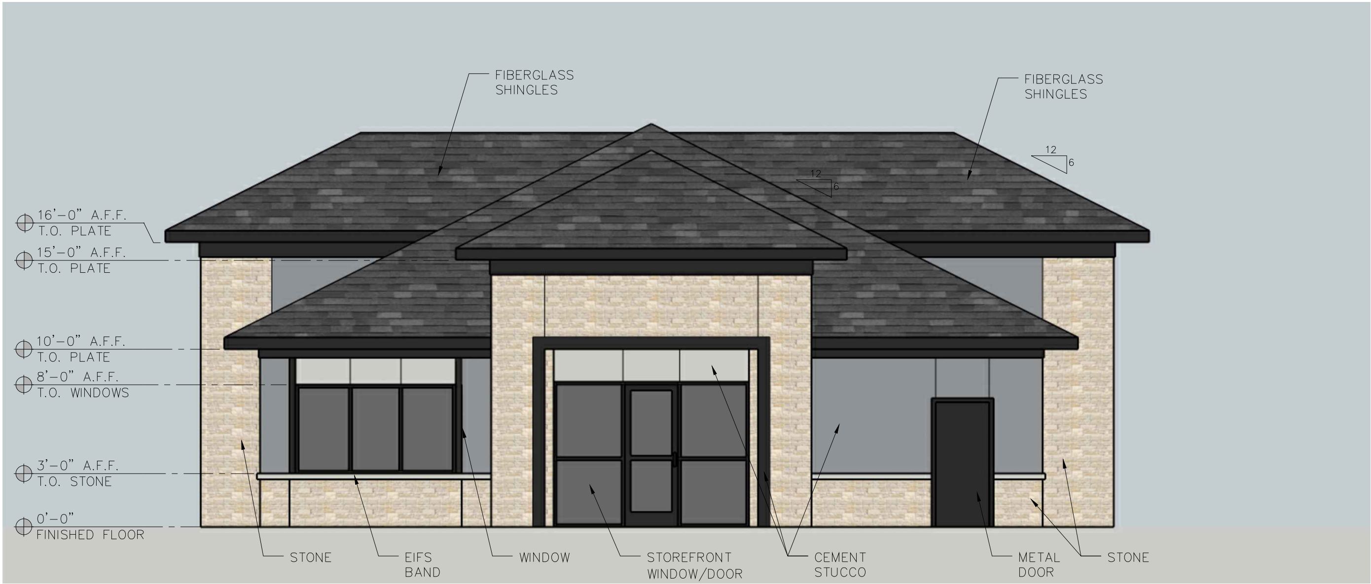
1 BUILDING B - EAST ELEVATION
