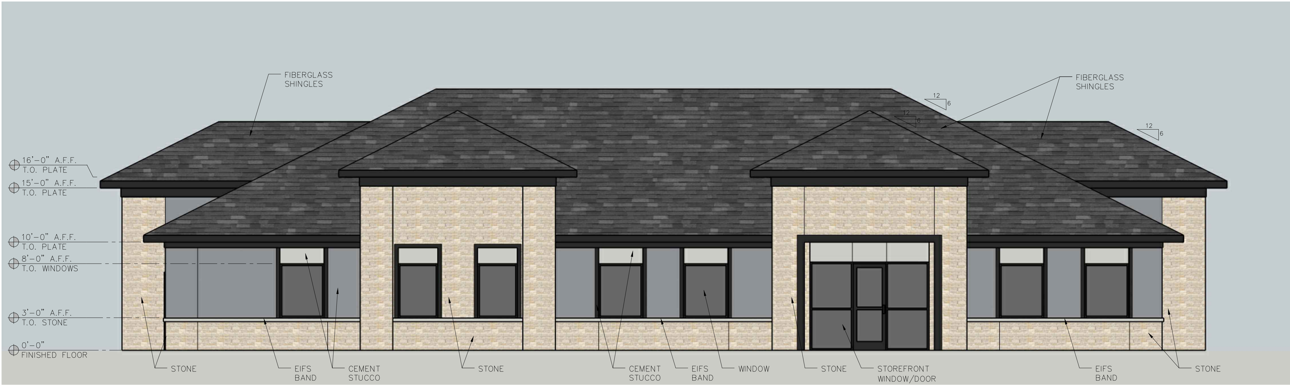
2 BUILDING A - NORTH ELEVATION
