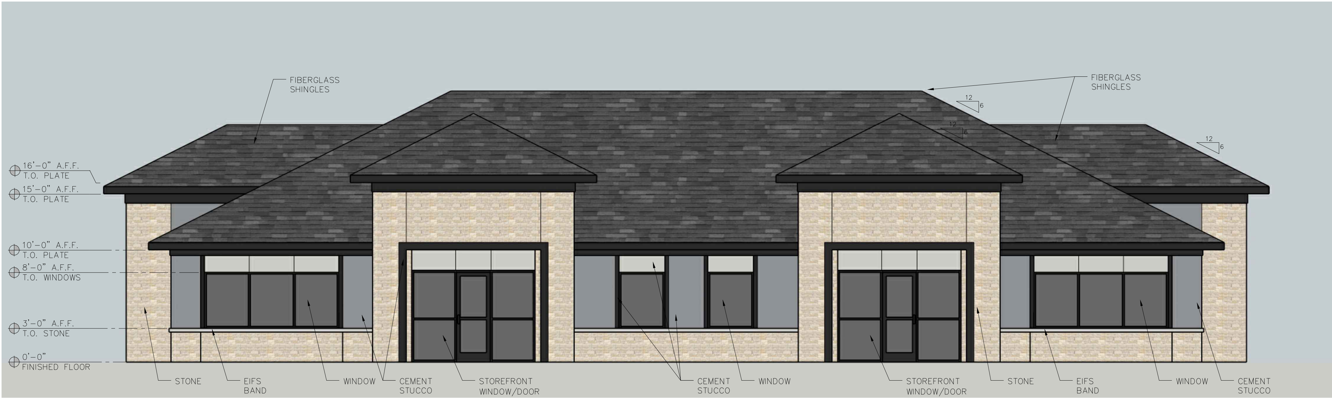
2 BUILDING A - SOUTH ELEVATION SCALE: 3/16" = 1'-0"
