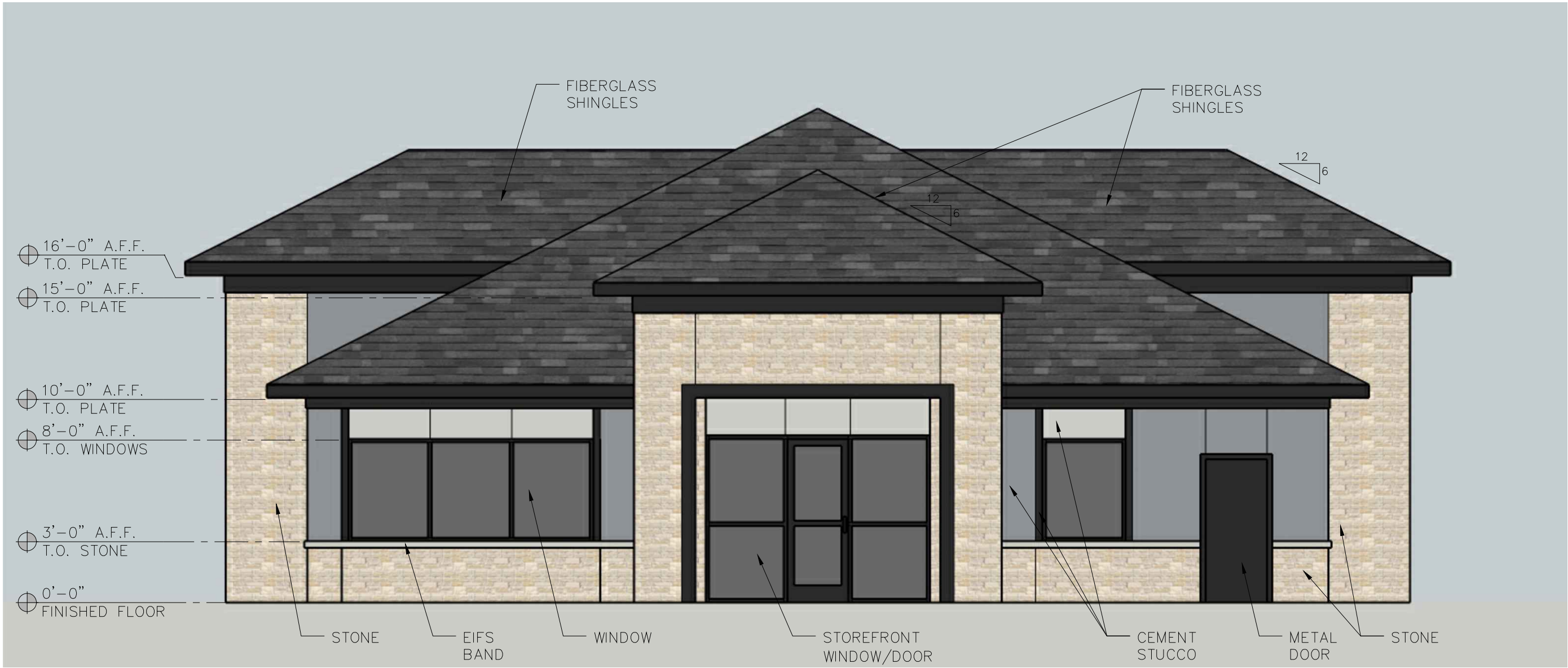
1 BUILDING A - EAST ELEVATION
