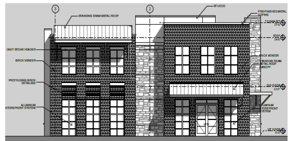
1 BUILDING 1 - NORTH ELEVATION SCALE: 1/8" = 1'-0"
