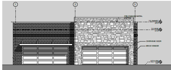
3 BUILDING 2 - SOUTH ELEVATION SCALE 1/8" = 1'-0"
