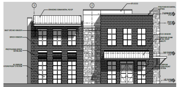
1 BUILDING 1 - NORTH ELEVATION SCALE: 1/8" = 1'-0"
