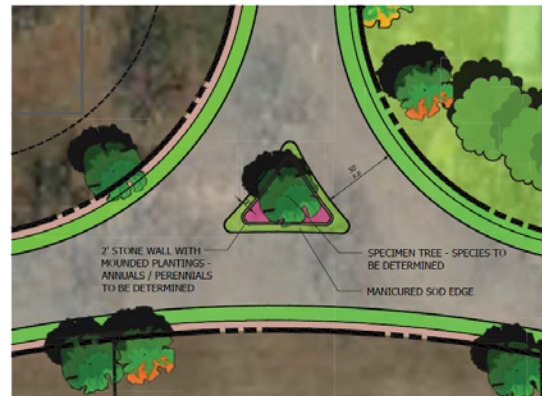
INTERSECTION STREET ISLAND DETAIL (TYP)
